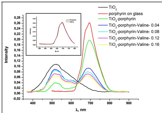
Fig.5.PL spectra of the TiO<sub>2</sub>-porphyrin sensor measured at different concentrations of Valine
