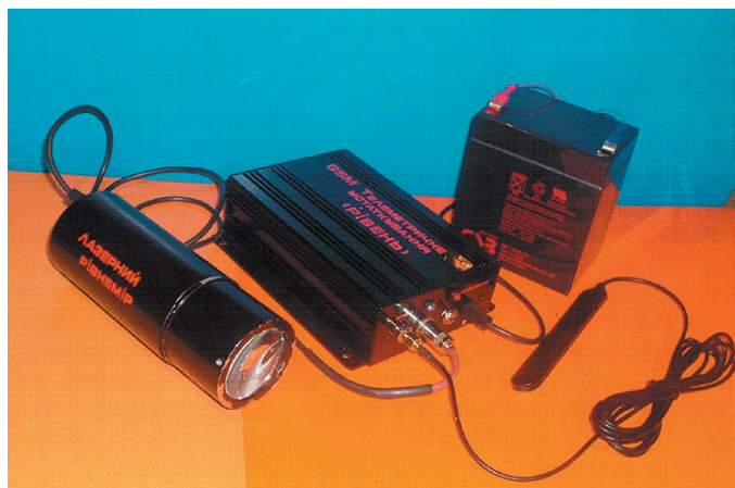
Fig. 3. A photo of the prototype of hydrometric station equipment.
