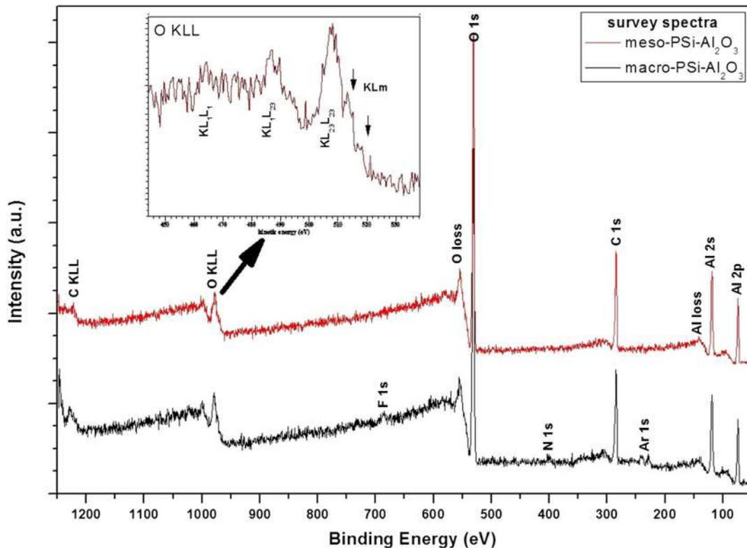
**Fig. 3.** XPS survey spectra of the meso-PSi- $\text{Al}_2\text{O}_3$  (red curve) and macro-PSi- $\text{Al}_2\text{O}_3$  (black). The main core levels are labeled. The data are normalized to each O1s peak maximum and separated vertically. (For interpretation of the references to colour in this figure legend, the reader is referred to the web version of this article.)
