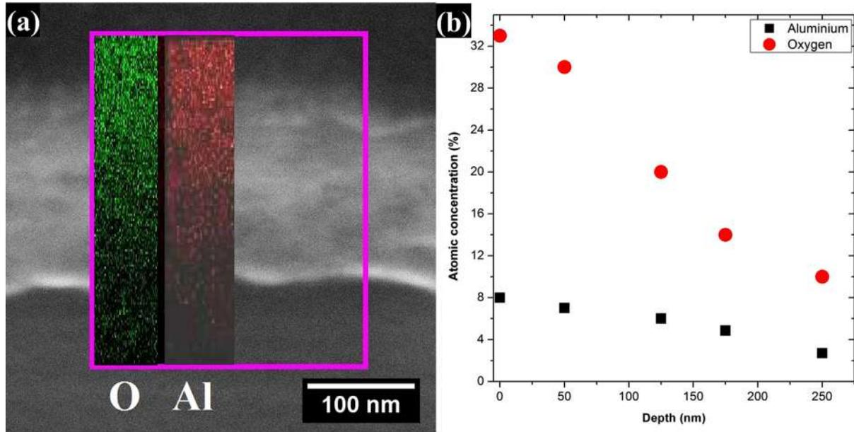
**Fig. 2.** (a) EDX elemental mapping of macro-PSi surface after 150 ALD cycles; (b) the concentration-depth profile of aluminum and oxygen for  $\text{Al}_2\text{O}_3$ -macro-PSi. Estimation was based on the SEM-EDX line scans of the sample cross-section prepared by FIB.
